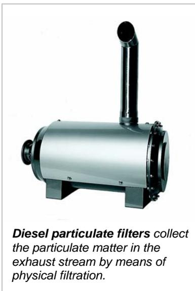
All types of filters have a finite capacity. DPFs are no different and must be cleared of the accumulated DPM, either at regular intervals, or during operation. Failure to do so will eventually cause the filter to block. This can damage or destroy the filter and may also damage the engine due to increased backpressure.
